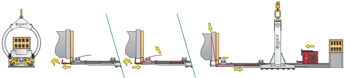
**2** Pull the tubesheet with rope
