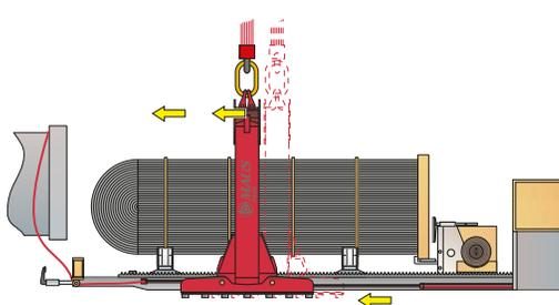
**6** Release from shell and depositing on ground using a crane
