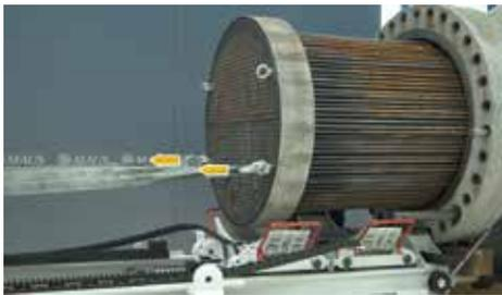
Pull the tubesheet with rope **2**
