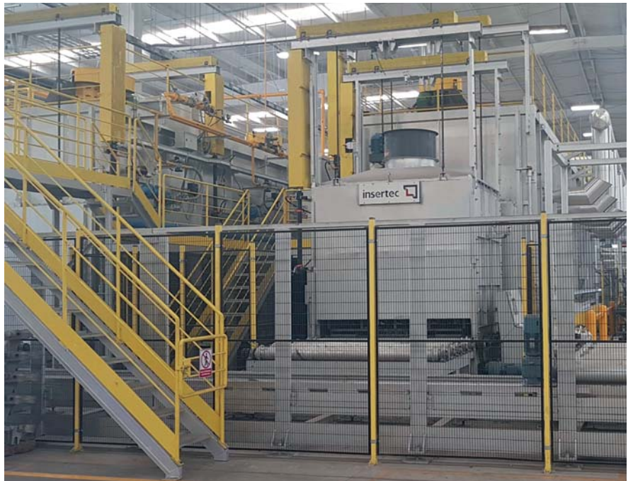
✎ T6 roller type continuous furnaces (T4, T5, T6 & T7 treatments), Intertec. Used in the automotive, railway, power generation and aerospace industries.
