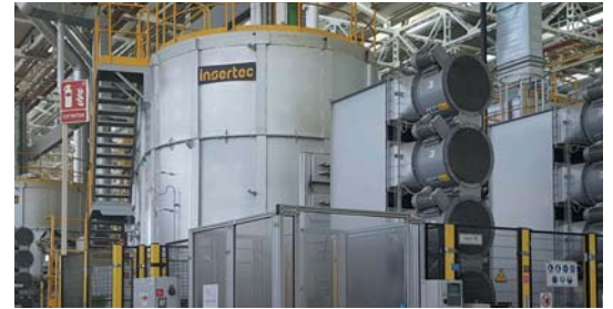
➤ Rotary hearth furnaces, Insertec. Heat treatment close cells for T5, T6.
