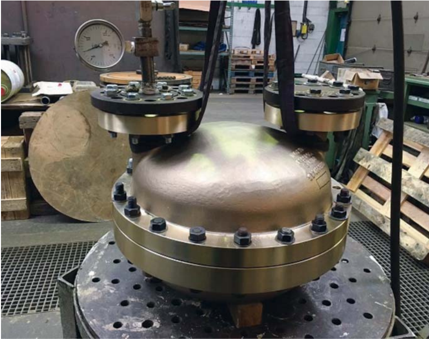
Figure 3: Example of Hydraulic pressure test.
