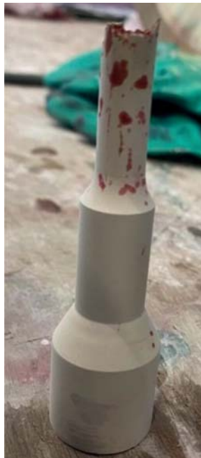
Figure 7: Dye penetrant test showing directional crack.
